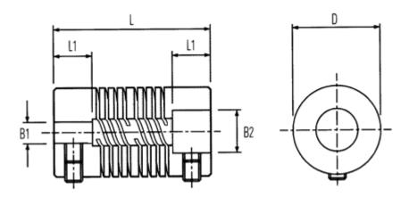
B1: Pre-drilled = 10.0B2: Pre-drilled = 16.00 D = 50.8 L = 95.3 L1 = 25.0 Max angular displacement = 0.90 Max B1 & B2 = 28.00
